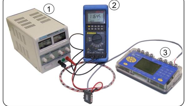
**NOTE** Programming of the temperature range can be made using resistances of precision with a fixed value which simulates values of Pt100 sensor (see table below of Pt100 values).
