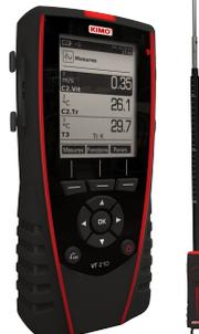
**VT210 + SMT 900 probe** (telescopic multifunction probe of air velocity, relative humidity and temperature)
